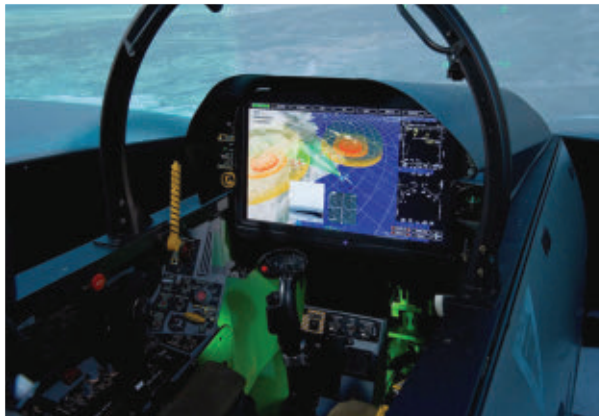
The Advanced Crew Station on the F/A-18 Super Hornet will contain a high-definition, touch-screen display that enables aircrew to view and manipulate information.
